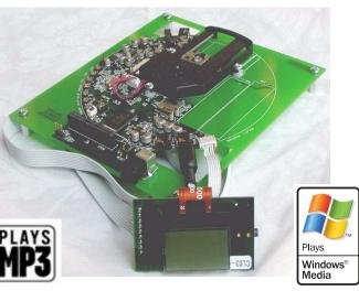
The CRD7410-HE is powered by the highly integrated Cirrus CS7410 solution for CD/MP3/WMA players. The CS7410 integrates microcontroller and DSP capability into a single device to provide a highly cost effective and compact solution for this exciting new class of consumer electronics products.
